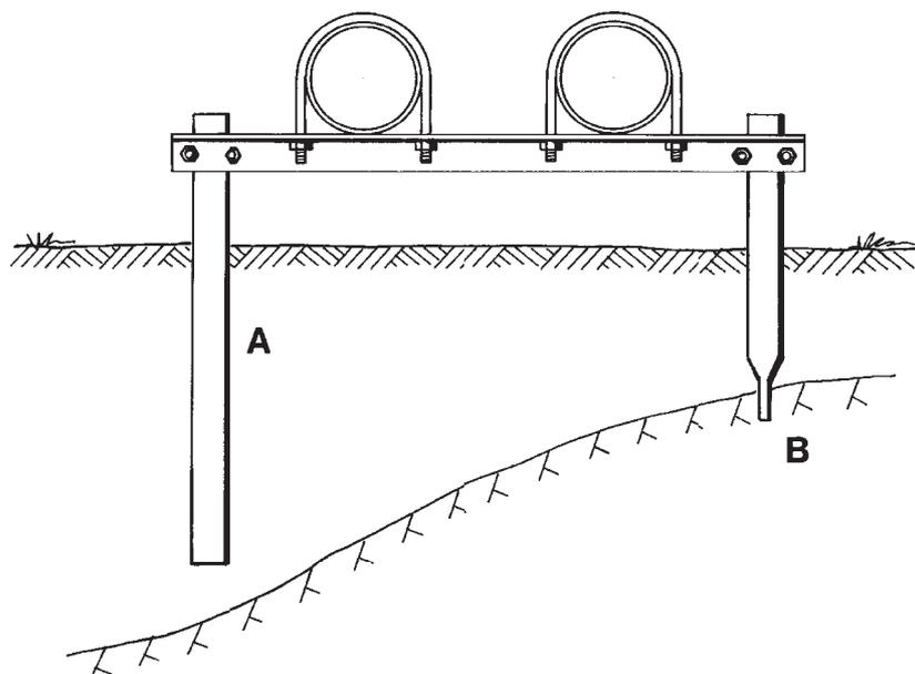
Figure 22. Compressed air system above ground. A=soil. B=rock.
