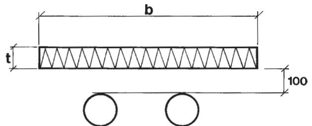
Figure 11. Horizontal insulation of pipeline.
