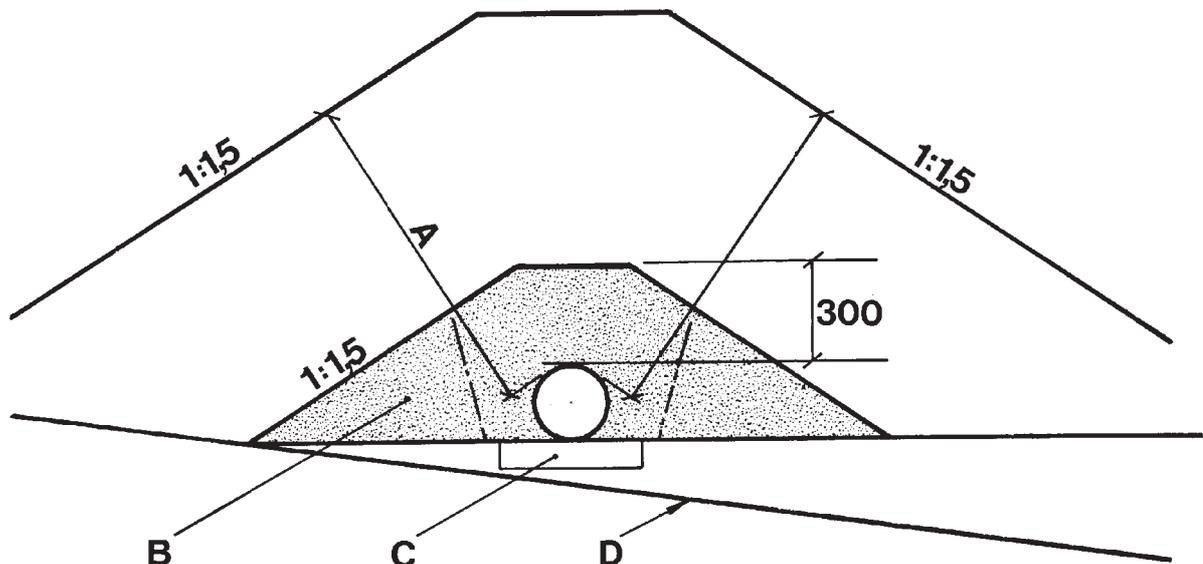
Figure 21. Surrounding fill for embankment. The fill for the embankments should be done with material from group 1, 2 or 3a table C/1 (appendix 1). A=required cover. B=surrounding fill. C=pipe bed (if required). D=existing ground surface.
