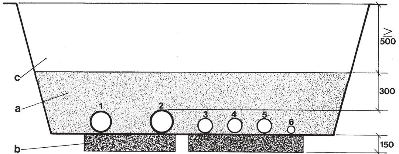
Figure 1. Example of a pipe trench cross-section that shows the pipes internal placement.
