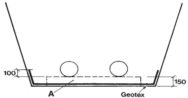
Figure 4. Material separating layer in pipe trench. Geotextile should be of bruksklass 2 according to Vägverkets classification. A=pipe bed.
