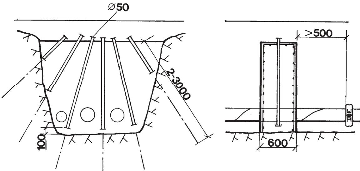
Figure 18. Seepage cutoff design of concrete in rock.
