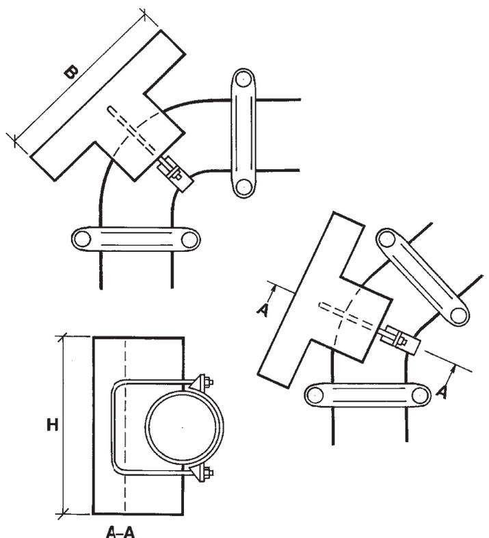
Figure 19. Bracing of pipes.
