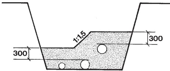
Figure 20. Allowed limit of fill surrounding the pipes in the pipe trench with lines at different levels.
