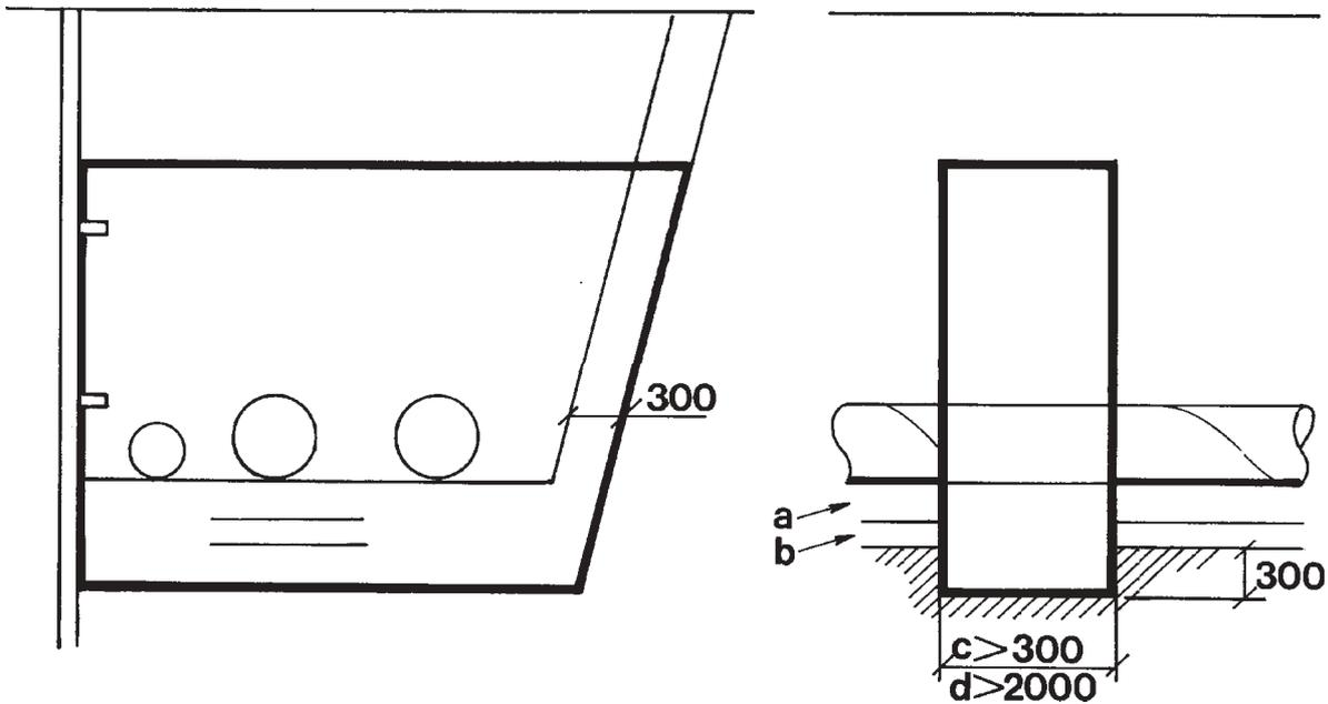
Figure 17. Seepage Cutoff Fill in Pipe trench. a=pipe line bed (as required). b=soil reinforcement (as required). c=thickness with concrete. d=thickness with dense soil
