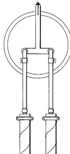
Figure 15. Low point manhole at the end of the line.
