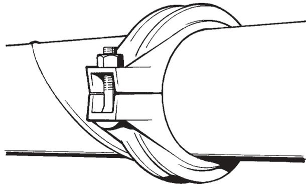
Figure 5. Alvenius quick couplings and pipes.
