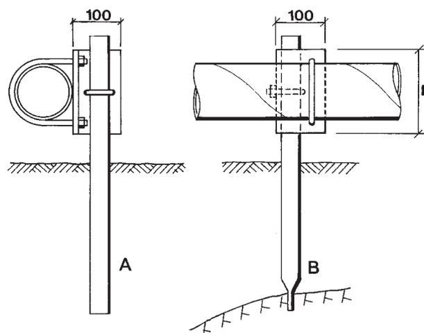
Figure 23. Fan system above ground. A=soil. B=rock. H:designed to fit the pipe dimension.
