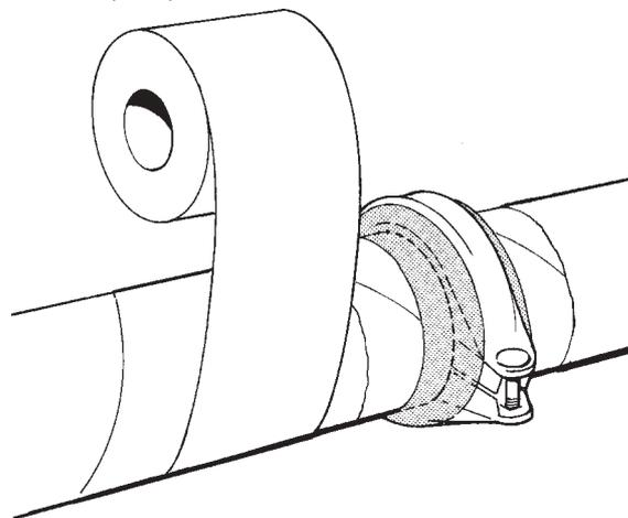
Figure 16. Triangle-putty is placed in the joint between pipe and coupling. Denso tape is wrapped around the coupling and at least 50mm (2") out on the pipes bitumen treatment.
