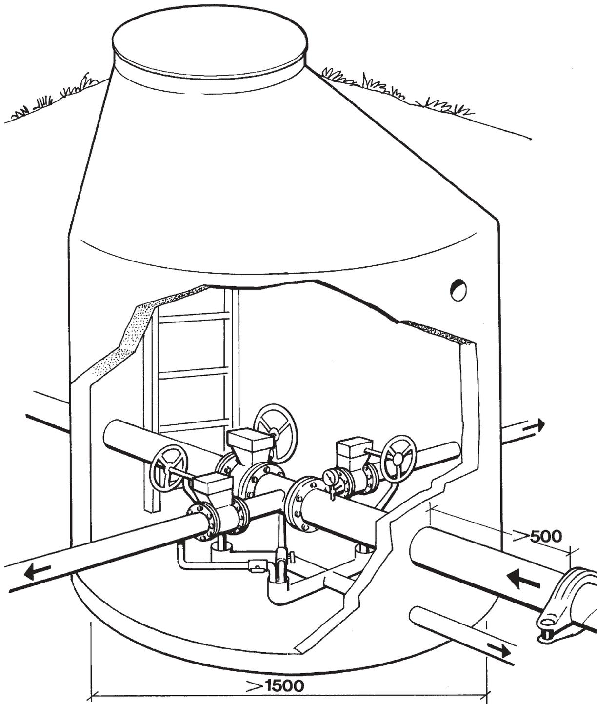
Figure 12. Sectioning manholes
