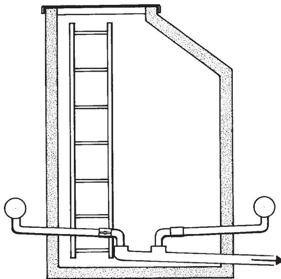
Figure 14. Low point manhole within the system
