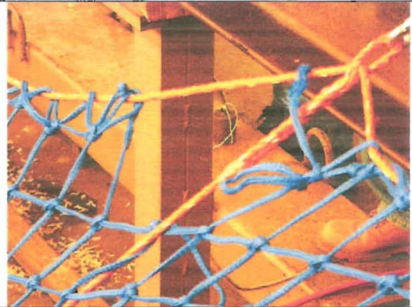
6. Impact test net sample 1 damage recorded
